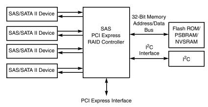
Figure 1.2 shows an example of a SAS RAID controller configured with an LSISASx12 expander that is connected to SAS drives, SATA II drives, or both.
